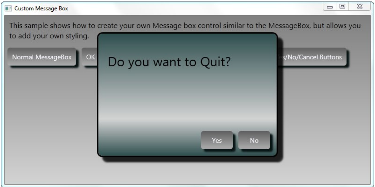
Figure 2: Creating your own dialog from a Window, a Text Block and a custom button control.
